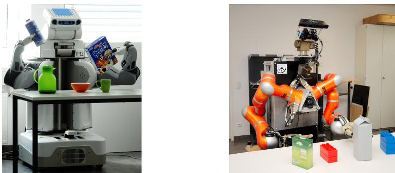
Figure 1. Different objects mostly require different grasping techniques and may not obstruct each other when placing them.
